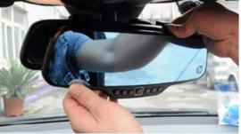
Pull up the extendable rod of the dashcam and fix it to the rear view mirror
