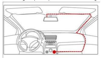
1. Connect one end of the car charger to the USB connector of the camcorder.
